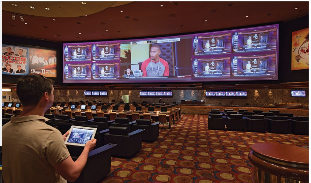
Operating the system via the iPad. Complete control including source preview is provided.
